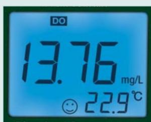
Large blue backlit dual LCD display with calibration and memory indicators
