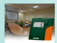
The Extech CO30 displays Carbon Monoxide (CO) concentration, Air Temperature, and Relative Humidity. Programmable audible alarm, with high decibel beeper, sounds when CO concentration rises to unsafe levels. Can be wall mounted or used on a desktop close to areas of concern.
