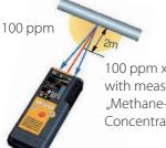
00 ppm x 2m = 200 ppm xmwith measured LMm called "Methane-Column Density" Concentration x Density
