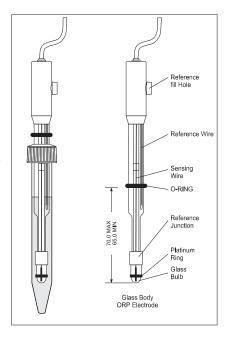
than  $2\frac{1}{2}$  cm (1") below the fill hole, add **MA9011** 3.5M KCl Electrolyte Solution. For faster response, unscrew the fill hole screw during measurements.
