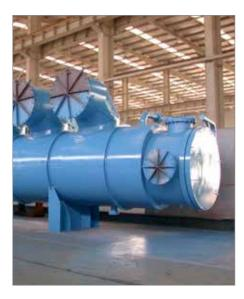
In heat exchanger equipment, flanges and bolts tend to expand and contract. The compressive force is typically increased to counteract the effects. As a result we have a full range of materials reducing the need for over Torquing.
