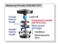
Optionally **GABOMETER®** systems can be upgraded for Fatigue tests in tension, compression and shear mode. Simultaneously, visco-elastic properties like E', E", E\* and tan delta can be determined (option). Samples and components can be tested within a frequency range from 0.01 Hz up to 100 Hz.
