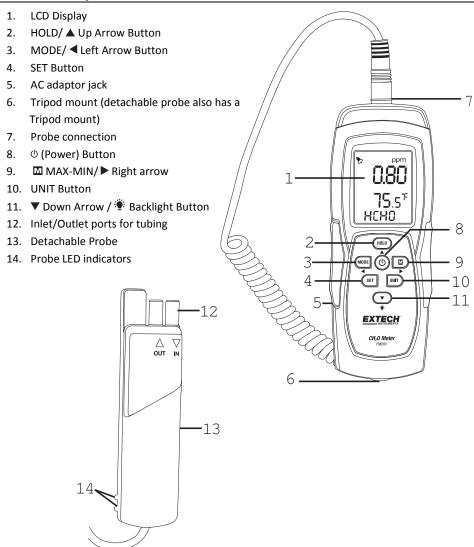
**Note**: Battery compartment located on back of the meter. A tripod mounting port is available on the back of the external probe.
