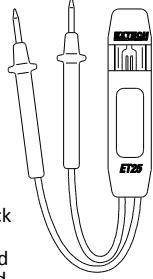
**2-wire AC Outlets and Cords:** Insert probes into both slots of the receptacle. Tester will glow on a live circuit. To determine hot wire, insert one probe into one of the slots and touch the other probe to the metal mounting screw or metal plate. If the screw is grounded, the tester will glow when connected to the hot wire. The other slot is the neutral.
