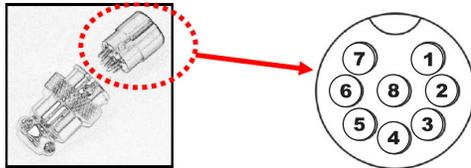
Note: Pin numbers are marked on the black area of the socket
