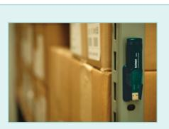
Monitors Temperature level in a warehouse or storage room.
