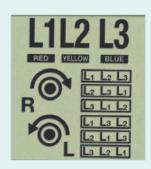
Easy to read graphical multilined LCD displaying phase orientation and showing which three phases is live
