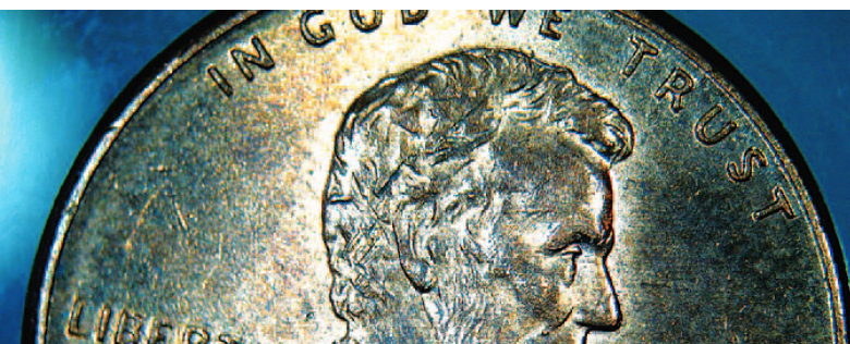
Stage 3 incident light: the lower two LEDs light finely structured objects from a low level, increasing contrast.
